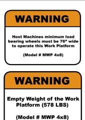
One each on the back of each MWP 4x8 Work Platform
