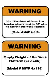
One each on the back of each MWP 4x116 Work Platform
